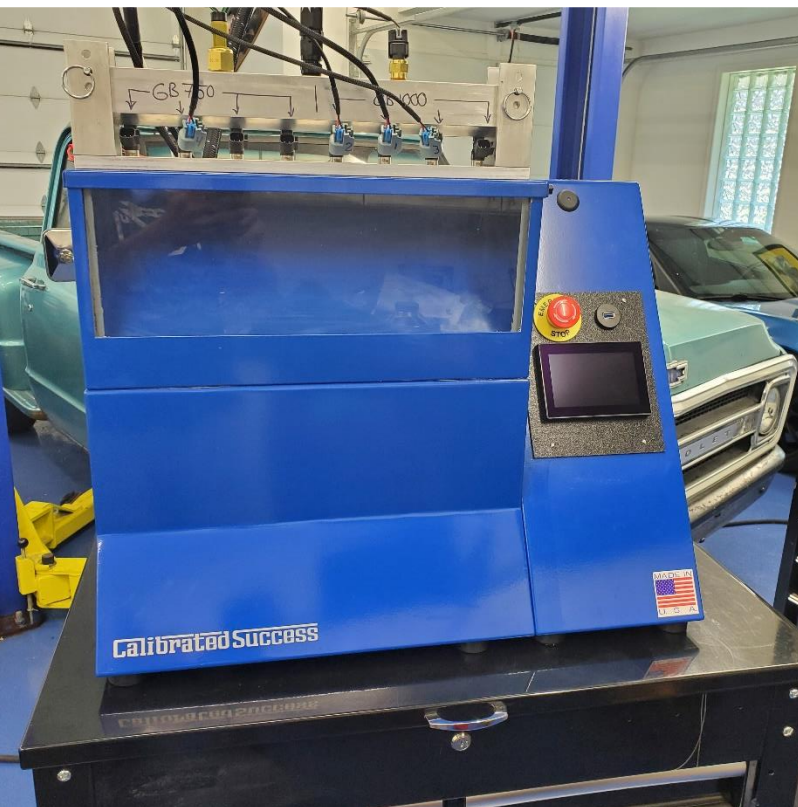
There's more to injectors than just a static flow rate. Testing them across a wide range of pulse widths exposes some interesting information that the ECU needs for complete control.
