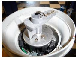
Perhaps the most limiting factor of running a single coil and distributor is that this one coil must charge and discharge between every single cylinder firing event on the engine. At 6000rpm, the engine completes it full two rotation cycle every 20ms. This leaves only 2.5ms to *charge and discharge* the coil between events on a V-8.
