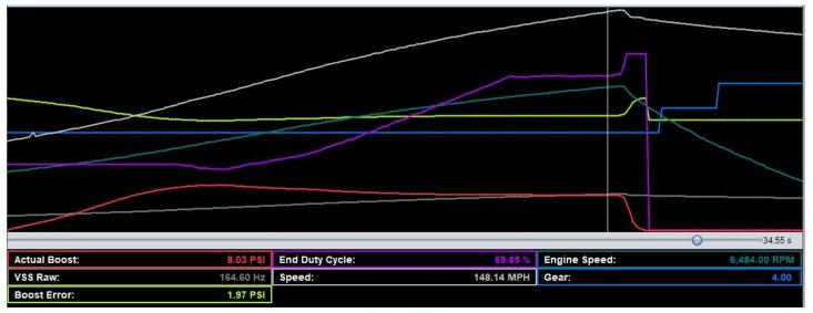
Unless we tighten the gates even further (risking overboost at 3500rpm), we will have to live with 8psi up top. With the calibration cleaned up, this new boost level was good for 607rwhp, an increase of 63rwhp from our baseline. The difference between the two runs is typical of a good dyno tuning session on a boosted car.
