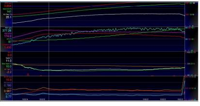
**HALF** of the 2psi/thread we expected from our earlier shop measurements, so the backpressure effect is not to be ignored in this case. We crawled under the car on the dyno and put another complete turn into them.
