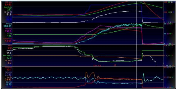
slightly more power with cooler inlet temps. The dyno reported just shy of 650rwhp with the ethanol blend in our final run, which correlates with our airflow numbers indicating north of 700hp at the flywheel.
