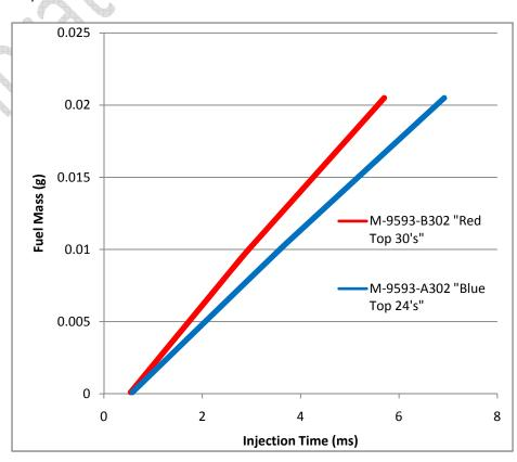
injector opens at all and fuel can begin to flow. A more careful look also shows how that the slope changes slightly with time for both injectors. This is a result of the non-linear flow of fuel through the holes in the injector. More on this later...
