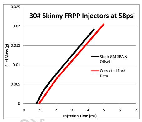
shift at the upper end. Below 2ms we also see that the nonlinear flow region is mismatched. The real solution here will be to knuckle down and do the homework to convert the known good Ford data into GM units so that the PCM can accurately deliver the proper fuel mass.
